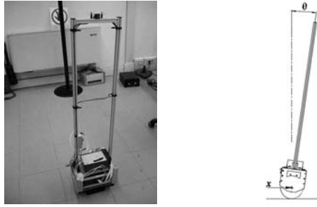
Fig. 1 The MWP robot Tilty and its degrees of freedom
